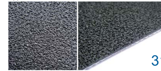
Name:Sandblast Code:31 Thickness:0.2mm Width:2000mm Property:Non adhesive surface, medium friction Application:Logistic, Treadmill belt, Roller wrapping
