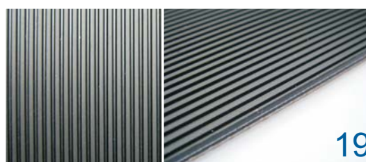
Name: Longi rib Thickness:0.7mm Property:Incline conveying, easy clean Code:19 Width:2000mm
